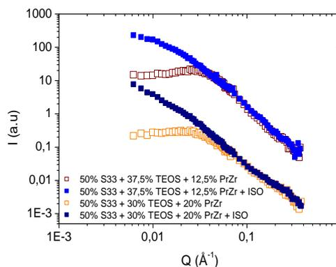
Figure 3 shows the SANS intensity obtained from samples with 50%PDMS and varying contents of TEOS and PrZr prepared with and without further addition of isopropanol. It was observed that the further addition of isopropanol in the preparation stage causes the inorganic fractal structure to extend over a much larger volume in the samples so prepared. This effect needs further investigation and work is in progress.
