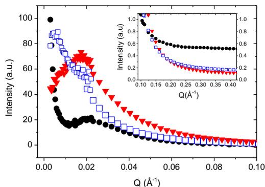
Figure 2 shows Small Angle Neutron Scattering (SANS) data for the 20%PDMS+73%TEOS+7%PrZr sample dried at room temperature ( $\bullet$ ) and after heat-treatment at 450 °C ( $\square$ ) and 600 °C ( $\blacktriangledown$ ). The insert shows the intensity at large  $Q$  before subtracting the incoherent scattering.
