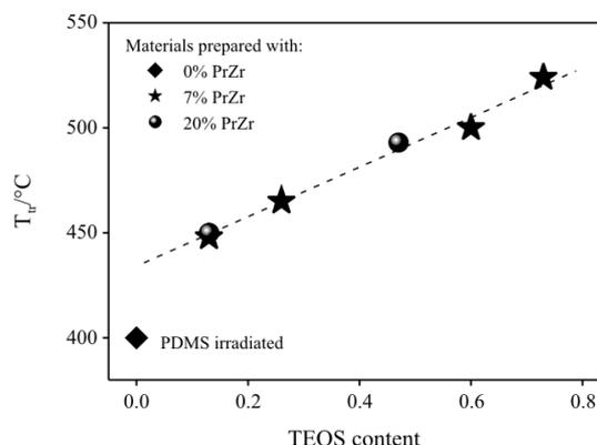
Figures 1 show the behaviour of the hybrid material rupture temperature,  $T_{tr}$ , which is associated to the breaking of the polymer chains into volatile fragments and marks the rupture of the structure. It was found that this temperature increases linearly with the TEOS content in the hybrid materials prepared with PrZr.
