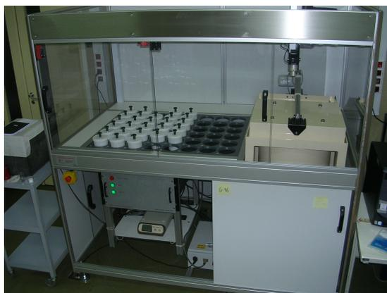
Samples can be positioned at different distances from the germanium detector by placing rings. Gamma spectra in digital form enter the  $k_0$  IAEA program for direct calculation of the concentrations. A Partisol Plus sequence air sampler was also acquired to collect
