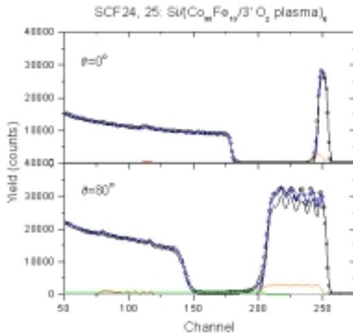
Fig. 2. RBS spectra taken at normal incidence and at a  $80^\circ$  grazing angle of incidence of a Si/(Co<sub>90</sub>Fe<sub>10</sub>/3' O<sub>2</sub> plasma)<sub>6</sub> sample.
