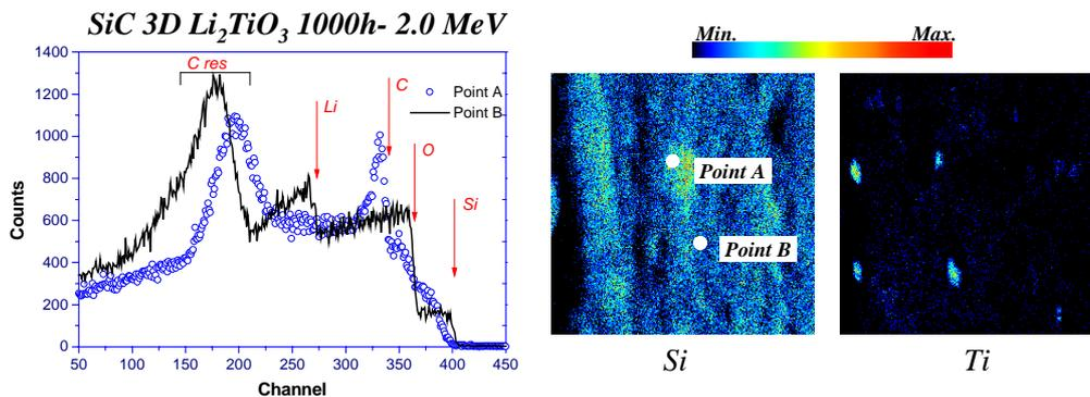
Figure 1. 500µm<sup>2</sup> scan elemental maps of Si and Ti for the SiC sample exposed during 1000h to Li<sub>2</sub>TiO<sub>3</sub> showing the formation of Ti precipitates. And RBS spectra from points A and B.
