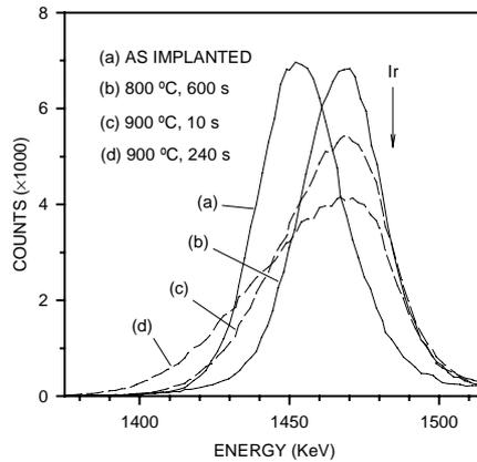
Fig. 2 - Ir-related RBS signal of samples annealed at different conditions.
