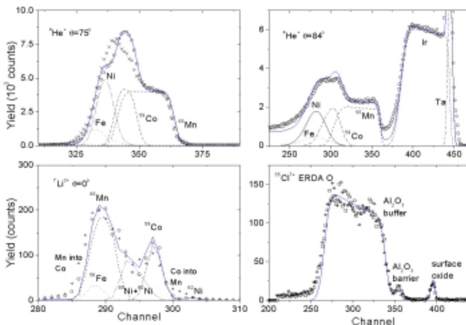
Fig. 1. RBS, heavy ion RBS and ERDA data for a spin valve structure as deposited (circles) and annealed (crosses).
