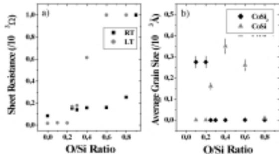
**Fig. 4** (a) Sheet resistance values for samples implanted at 350°C (LT) and at room temperature (RT). (b) Average grain size for LT samples vs. O/Si ratio in the buried porous layer.
