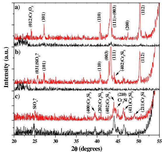
**Fig. 3** X-ray diffraction results for a) C6HT, b) C6OXHT and c) SOXHT samples (Cr implanted samples with increasing O/Si ratio in the porous layer). Lower and upper spectra correspond to as implanted and annealed (700°C, 90 min) samples, respectively. The peaks indicated simply by their lattice plane correspond to CrSi<sub>2</sub>.
