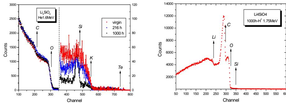
Figure 2. µRBS of Li<sub>4</sub>SiO<sub>4</sub> ceramic pebbles: Left) virgin and exposed samples analysis with 1.6 MeV He<sup>+</sup> beam show the formation of a Si surface layer; Right) RBS C signal is enhanced through the use of a proton beam of 1.75 MeV.
