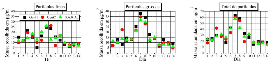
Fig. 1 – Gravimetric measurement of collected masses by the three samplers, S.A.R.A. being the automatic filter change system and the others two identical Gent PM10 samplers. Data are shown for fine particles (partículas finas), coarse particles (partículas grossas) and the sum of both (Total de partículas).
